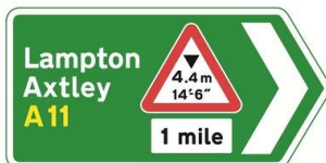
Primary route sign showing destination, road number and restriction
