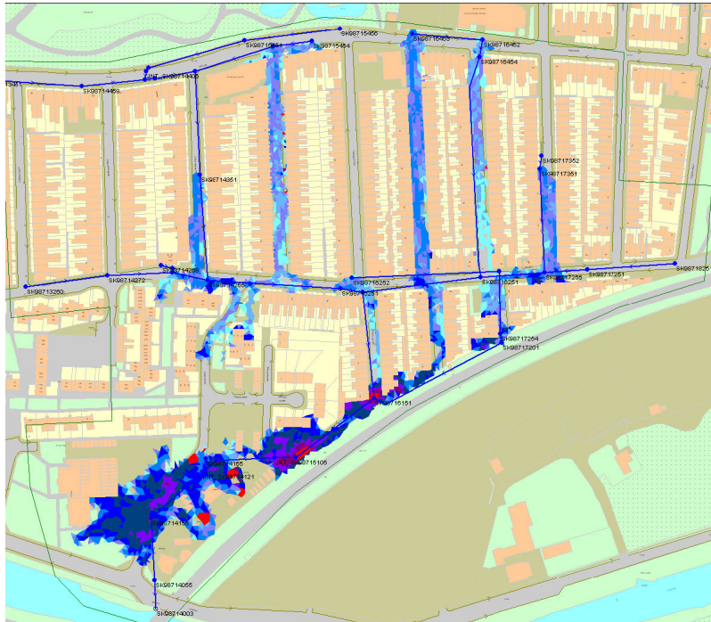
Figure 2.7 Routing of surface water in the Lincoln pilot study
