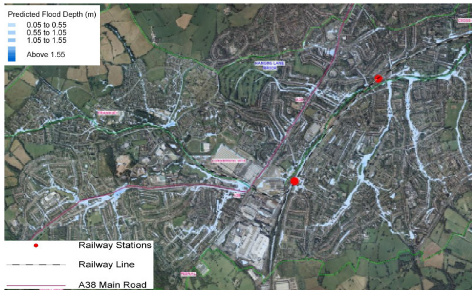
Figure 2.10 Predicted surface water flooding depths in Upper Rea catchment for 100 year event plus climate change
