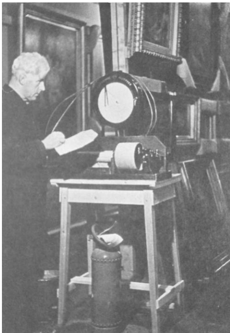
Fig. 2.6 – An hygrometer consisting of disc-type temperature recorder and aspirating system was used for monitoring the environmental conditions inside the repository (from Saunders 1992, p. 108)
