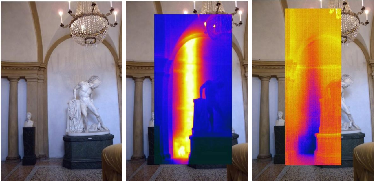
Fig. 4.3 – Thermography is used to analyse the effects of the historical heating system in winter and summer.
